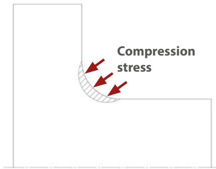
Figure 5 - Compression stress after deep rolling
