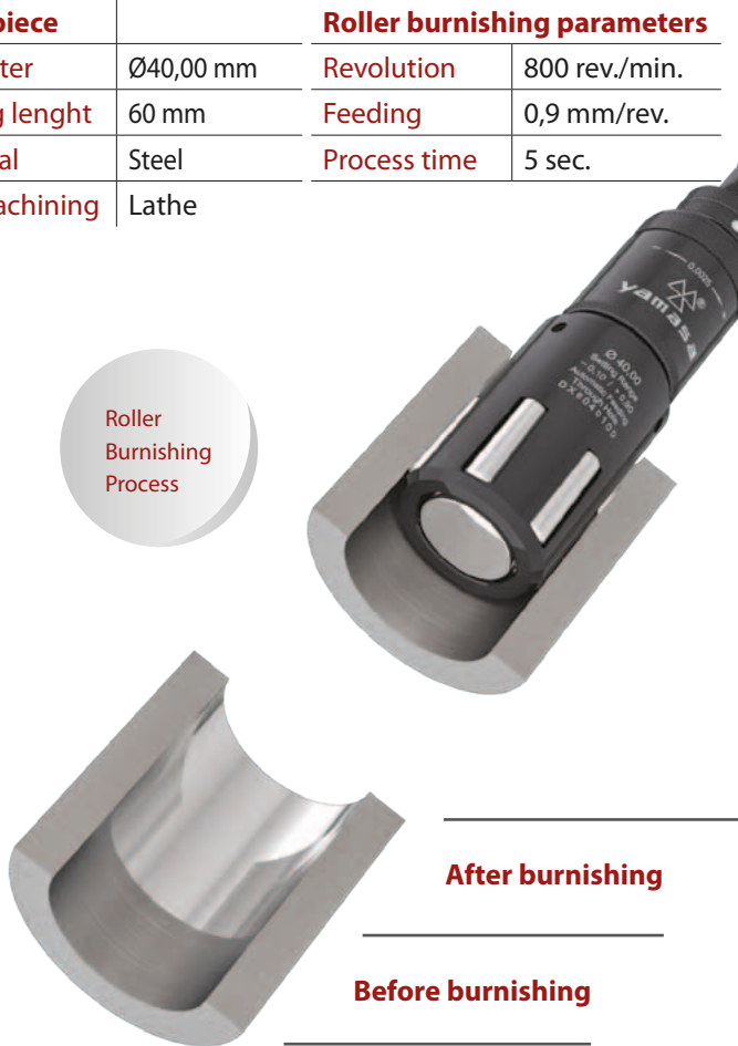
Figure 3 - Before and after roller burnishing surfaces
