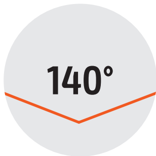
Affilatura frontale a 140°. 140° front sharpening.
